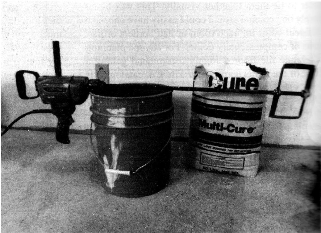
**Figure 22-4.** *Thin-set ceramic tile mortar.*
